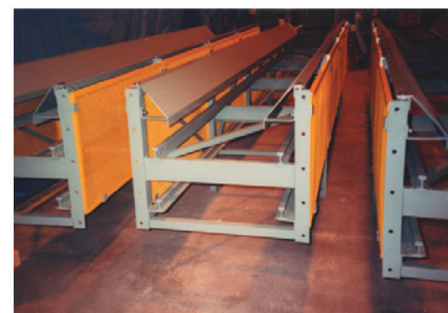
Open frame design with expanded metal guards
